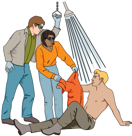
Figure 38-7 Use of a shower for flushing
